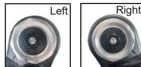
The force increases and the restoring damping force decreases for counterclockwise rotation (S direction). Adjust the left and right shock absorbers to the same damping force level.
