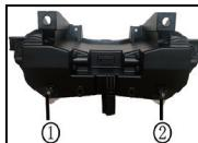
to raise the right low beam and high beam simultaneously.
