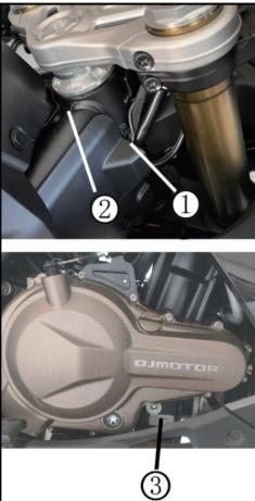
② Riveting position of product nameplate: left side of head pipe.
