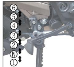
Because of the ratchet mechanism, it is not possible to raise or lower more than one step at a time.
