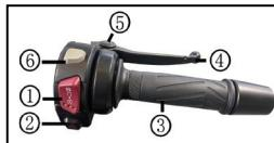
Turn the switch to "⊗" position: The motorcycle circuit is turned off, and the engine cannot be started.
